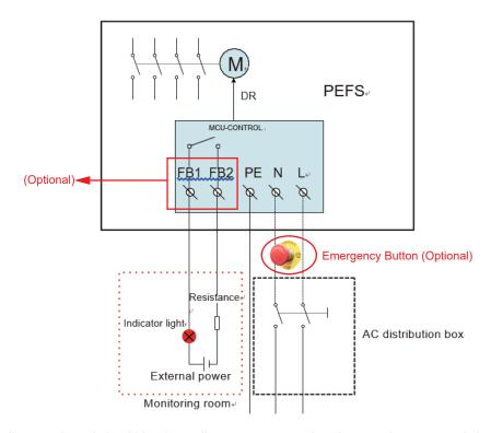
Resistor and indicator selected should be depending on power supply voltage and current, and should be less than 320mA
